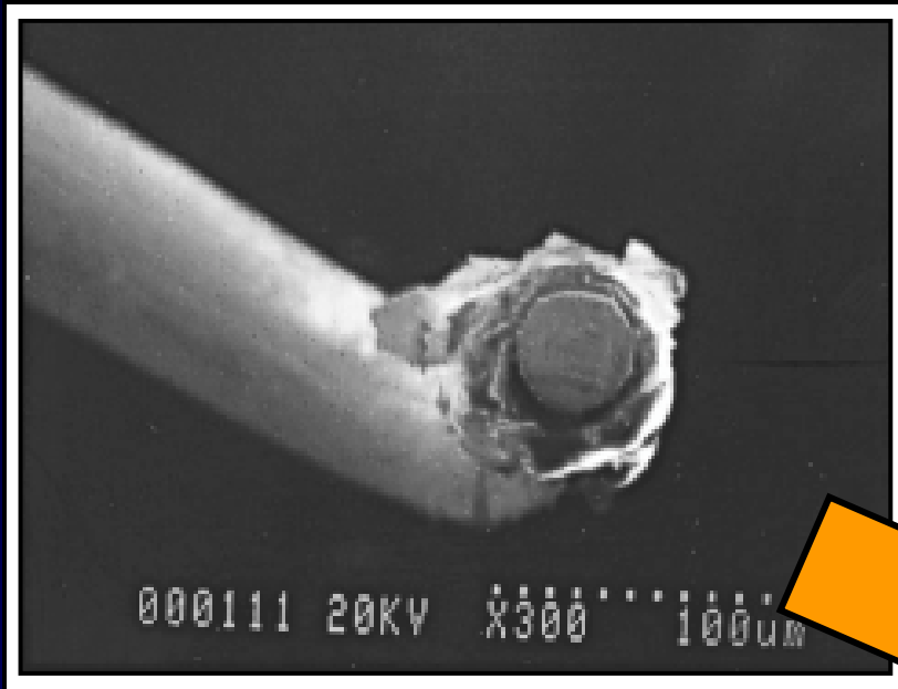
Cantilevered Probe Adherent Debris
