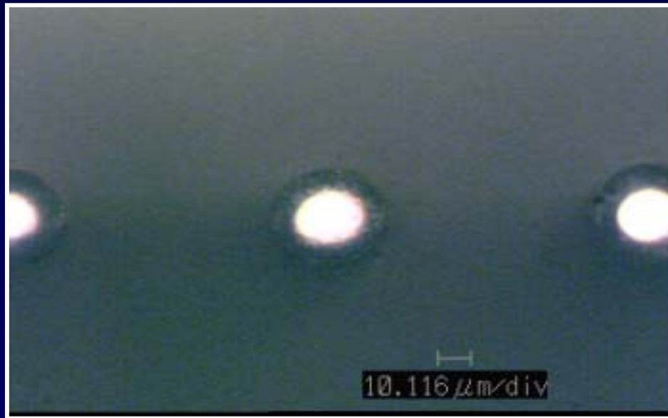
Probes after Non-destructive Cleaning (Mag: 150X)
