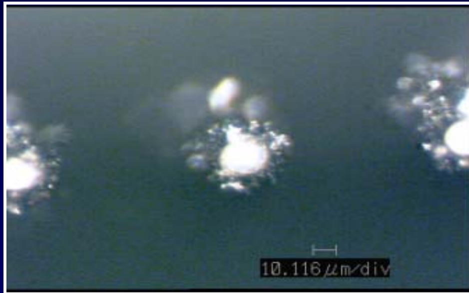
Probes after Touchdowns on Bond Pads (Mag: 150X)
