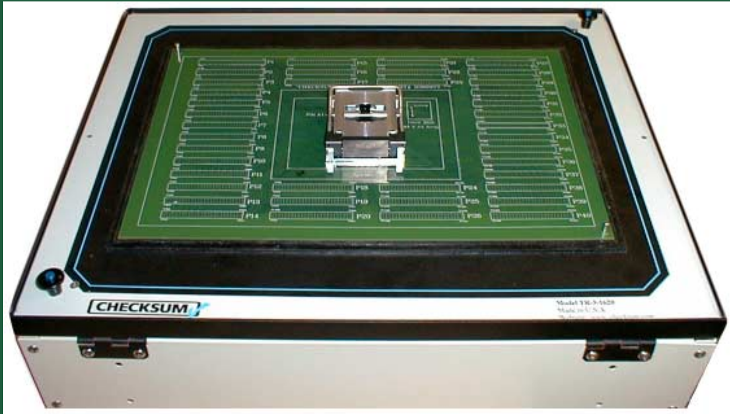
Load board on vacuum test head
