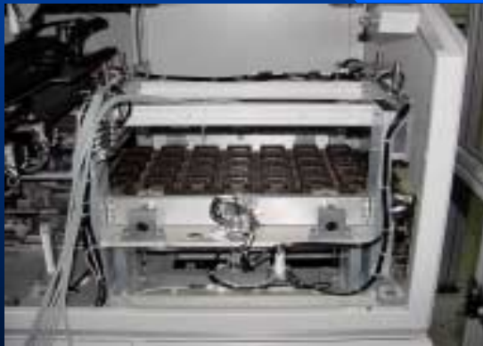
Loaded BIB is transported to 100% Board Check Station (BCS) module
