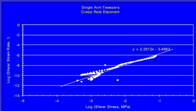
Figure 10. Shear strain rate vs stress for data from Finite Element Analysis for single arm tweezers. The slope, 2.2512 in the expression above for a best fit line is the stress exponent,  $n$  in the creep equation.
