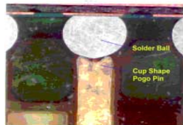
Fig 6. X-sectional view of a Socketed Package
